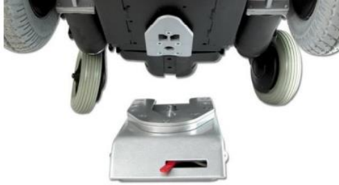
Docking station and docking plate on chassis
