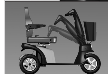
Folding down the steering column
