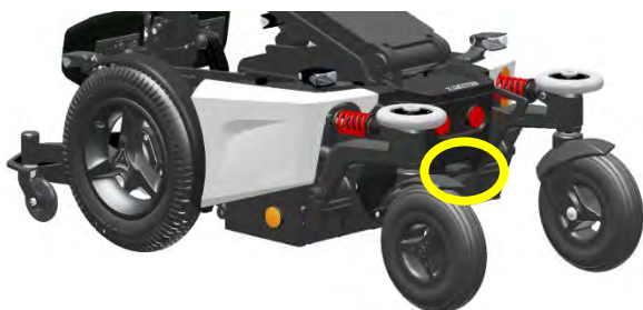
Position main fuse
