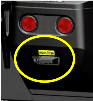
Place of the main fuse
