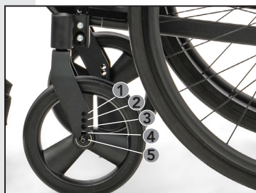
Positions 1 to 5 correspond to the height of the wheel in the clevis.
