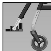
T3-B: 5 holes visible
