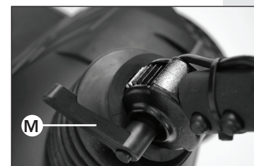
Folding down the steering column
