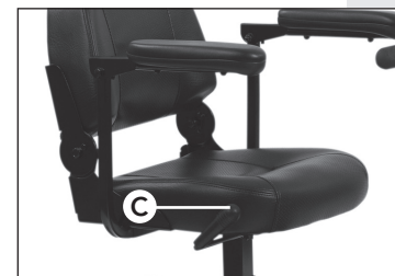
Removing the seat
