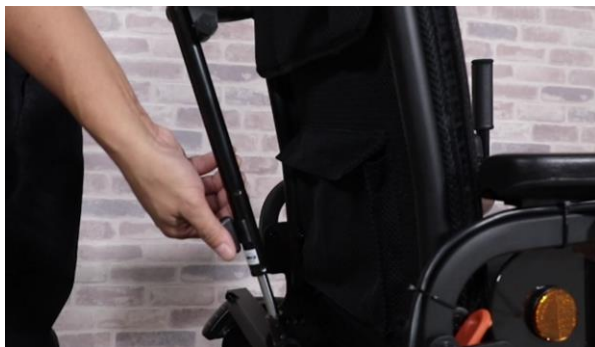
Push the recline lever on Sling Seat
