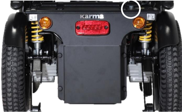
Circuit breaker location
