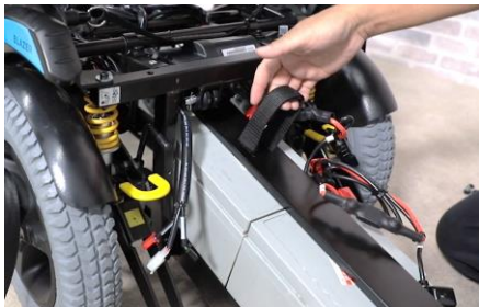
step 9. Use the rear and front strap to pull out the battery plate
