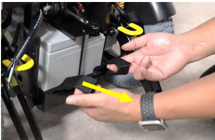
step 9. Use the rear and front strap to pull out the battery plate
